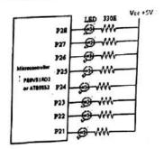
Figure 6.1 LED connections at port2
